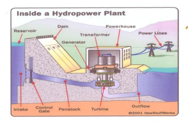
It's a general layout given by above. Hydroelectric Power Plants convert the hydraulic potential energy from water into electrical energy. The main component of this power station were Dam, Spillway, Penstock & Tunnel, Surge Tank and Power Station.
